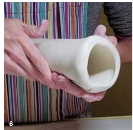
6 Roll the bottom edge of the pitcher body on a tabletop to form a rounded ledge.
