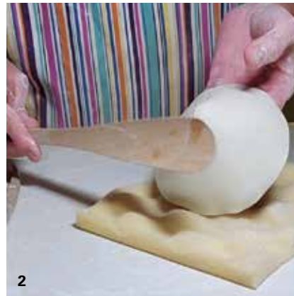
2 Compress the cone tip with a roller, then paddle it to avoid cracks forming.
